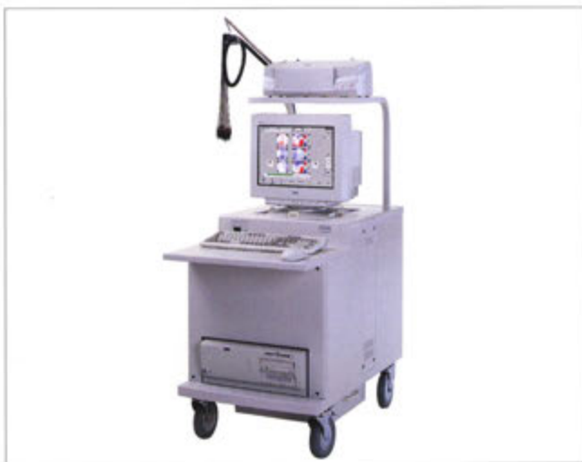
Fig. 1 General View of Optical Topography System (ETG-100)
