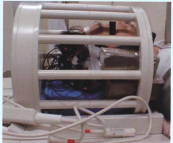
Fig. 3 Fibers mounted inside MRI coil for Optical Topography.
